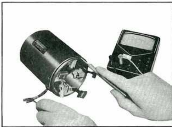
Fig. EE-59 Field Coil Tester Ground
