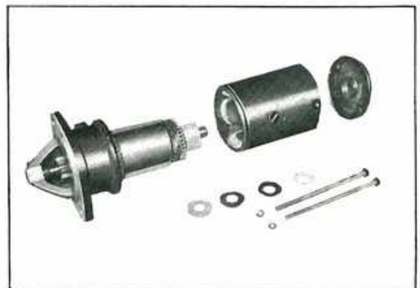
Fig. EE-54 Separating Yoke Ass'y and Armature Ass'y
